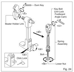
Reverse the previous sequence and attach the Spring Assembly, Beater Holder Link and the Beater to the Slave Side Pedal. Change the position of the Key Bolt as shown on the Uni-Lock Footboard Angle Cam for easier access when making Footboard angle adjustments (Fig.25). Your Slave Side Pedal is now ready to be used as a Single Pedal.
