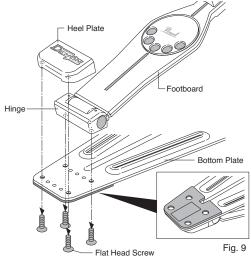
Lift the Footboard and remove the four 3-Piece Screws with the provided Multi-Function Drum Key or Allen wrench (3mm) as shown, and remove the Hinge from the Footboard (Fig.10).  $\swarrow$
