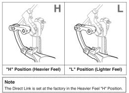
To change to a Lighter Feel, remove the Key Bolt with the Multi-Function Drum Key as shown. Move the Direct Link to the forward set of holes and re-attach the Key Bolt. To change back to a Heavier Feel, remove the Key Bolt and attach the Direct Link to the rear set of holes (Fig. 7-A, 7-B).
