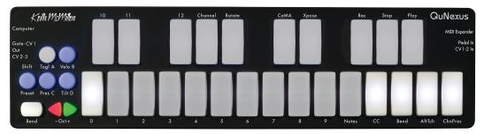
These key buttons act as toggles as well to turn Channel Pressure, Poly After Touch, CCs, and Channel Rotation on and off. Note that if you turn CCs off, all 3 possible CCs from Keyboard Layer will not output unless you turn them back on.
