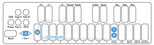
To **Transpose** the QuNexus, use the key labeled "Xpose" with the steps listed above. You can go up or down 11 semitones. If you are below 0 the - Oct button will blink; if you are above 0 the + Oct button will blink.
