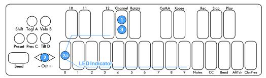
To set the **Pitch Bend** Range use the key labeled "Bend" with the steps listed on the previous page (shown below). You can go from 0 to 12 semitones. If it is set to 0, Pitch Bend will be disabled. The Bend Range will apply to the Bend Pad and also anything set to Pitch Bend in Keyboard Layer.
