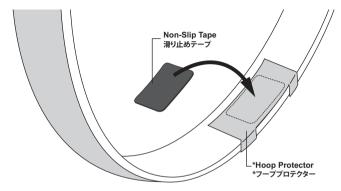
Apply the Non-slip Tape as shown if additional grip is necessary. Make sure that your pedal fits onto the hoop before applying the tape.
