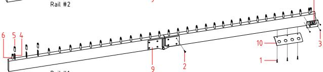
Rail #1 Pos# Cat# Description 1 PB124 Head tapping screw 2.9x19 mm, black 2 PB128 Cross recessed countersunk head tapping screw 3.5x20, black 3 PB141 Cross recessed panhead tapping screw 2.2x6.5, black 4 PM104 Gaf open 5 PM003 Rubber sleeve 12x10x23, black PM043 6 Cilindrical corner pen 7 PM106 Name plate Adams, gold Type plate Adams: Marimba Solist 8 PM115 9 PB717 Hinge for rails marima 10 PM056 Mallet holder for marimba / xylophone
