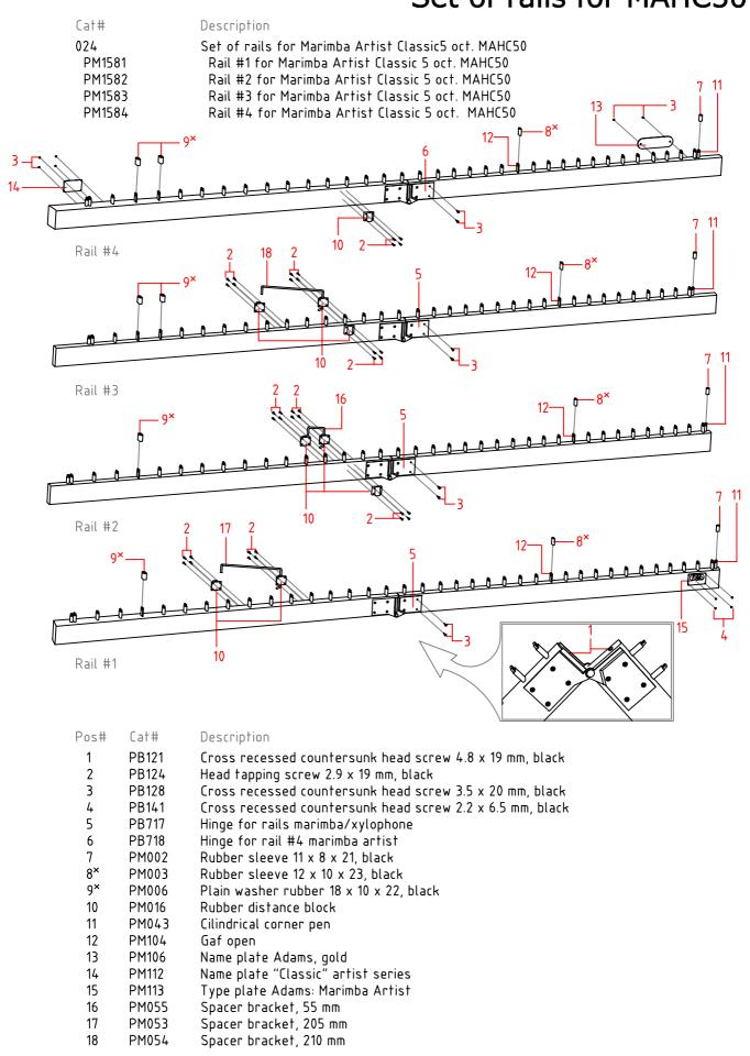
\* Pos #9 is only used at the places as drawn, for the rest of the gafs is used pos#8
